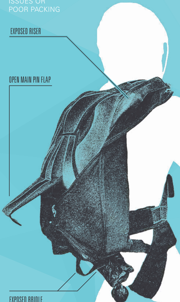
EXPOSED BRIDLE, LOOSE B.O.C. POUCH
