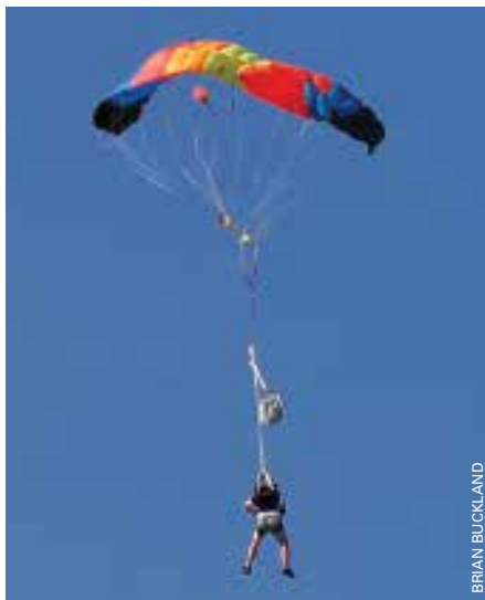
A jumper makes an intentional cutaway on a rig equipped with a United Parachute Technologies SkyHook.
