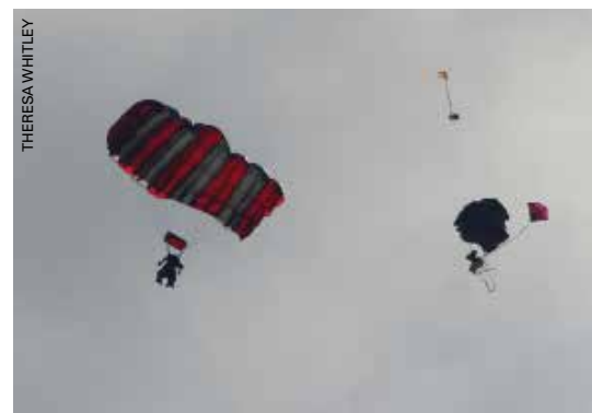
A tandem pair under its reserve flies away from a cutaway main canopy following an RSL-initiated reserve deployment on a Strong Enterprises tandem rig.
