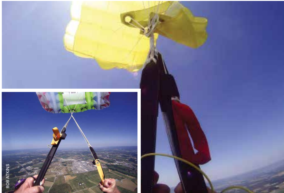
Jumper Bob Atkins, who was flying a Performance Designs Velocity 90 loaded at 2.5:1, cut away from a spinning malfunction. His rig was equipped with a United Parachute Technologies SkyHook MARD, which deployed his reserve, a Performance Designs PDR 113 loaded at 2:1.
